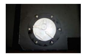
5. Fit tank breather to fuel tank using bolts provided. Carefully remove factory breather hose from fitting at fuel sender. Re-attach breather hose to fuel sender and roll over valve.
