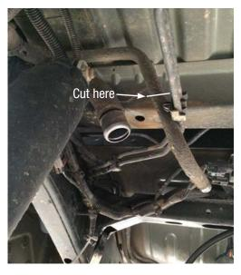
Cut straight piece of fuel filler hose as indicated in image.
