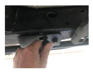
**9.** Feed nut plate on wire through the hole behind the front mount, align with chassis mount side hole and use M10 bolt to secure.
