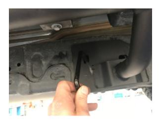
**8.** Secure front mount to underside of chassis using 2 X M12 bolts.
