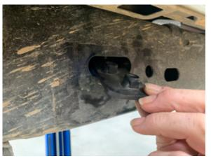
**6.** Lift side step into position locating the two body mount bolts and reuse factory nuts.
