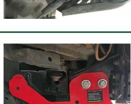
6. Using the last supplied long M12 bolt, pass through the rear most hole picking up the spacer / crush tube, secure with washers and nut.
