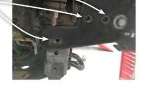
4. Place recovery point into position, and replace the 2 x bolts that pass through the chassis and leave loose.
