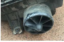
15. Refit air box to vehicle, attach to rubber joiner and secure with hose clamp provided.
