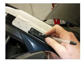
12. Install snorkel body to vehicle using M8 Nylock Nuts and body washers provided and attach to pillar bracket using M6 bolts and washers provided.
