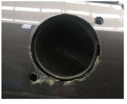
9. Using thread-lock screw 4 studs into the rear of snorkel body in position shown. Attach pillar mounting bracket loosely to snorkel using M6 bolts provided.
