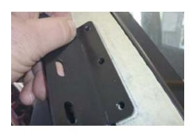
10. Hold mounting bracket against pillar in position previously marked and mark three mounting holes. Drill to 7.5mm
