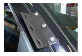
12. Install snorkel body with foam gasket to vehicle using M8 Nylock Nuts and body washers provided and attach to pillar bracket using M6 bolts provided.
