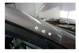
13. Install snorkel body top vehicle using M8 Nylock Nuts, rubber insulating washers, body washers and secure to pillar bracket.
