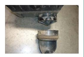
16. Using a grinder or file, remove all tabs from air entry snout on air box. Seal any holes in air box using sensor-safe silicone.
