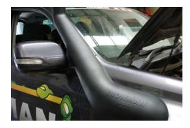
14. Feed rubber hose from engine bay through air entry hole in inner guard and attach to snorkel body. Secure using hose clamp provided.
