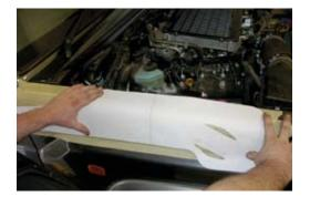
5a. For vehicle without factory snorkel cut two semi circles holes using a 89mm hole saw as shown.
