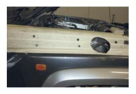
7. De-burr and rust-proof all holes (this applies to all holes drilled after this step).
