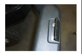
10. Hold snorkel in position on mudguard and mark position of upper mounting holes.
