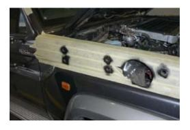
8. Apply rubber edging to large hole as shown.
