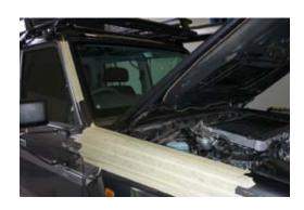
4 Hold template in position on the right hand mudguard and mark all holes and outer edges of two 'triangles' using a felt tipped pen or marker.
