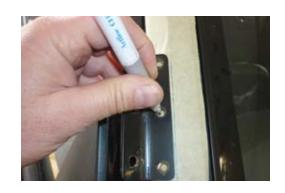
11. Remove snorkel body from mudguard and drill upper mounting holes to 7.5mm. De-burr and rust proof holes. Apply silicone to holes and insert mounting plugs.
