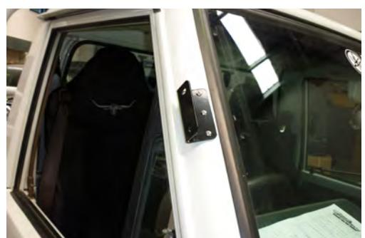
12. Attach snorkel body to mudguard using M8 Nyloc Nuts and body washers. Attach to pillar bracket.
