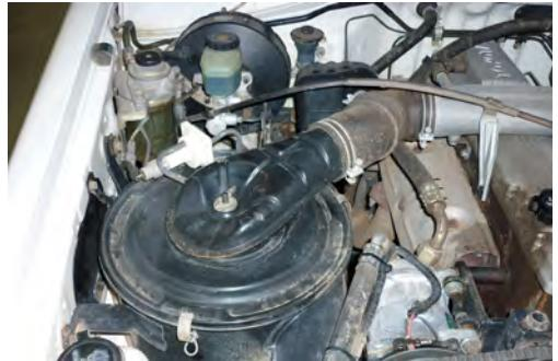
2. Remove air cleaner assembly, air intake duct to air cleaner, Landcruiser badge, plate from right hand inner guard and unbolt fuel filter assembly from inner guard.
