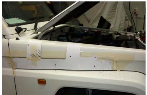
4. Tape template to mudguard making sure it is lined up with top of mudguard (bonnet opening) and rear of mudguard (door opening). Using a felt tipped pen, mark all holes through template onto mudguard. Remove template.
