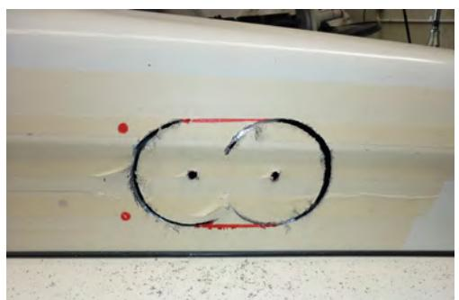
5. For snorkel outlet, using an 89mm hole saw cut two semi circles as shown. Mark a line between top and bottom of the semi circles and cut along lines using an air hack saw.
